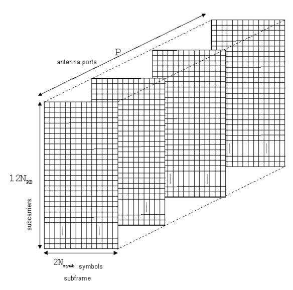
The rows of this array represent the subcarrier, while the columns map the OFDM or SC-FDMA symbols in the downlink and uplink respectively. The third dimension or plane represents the antenna ports. In the LTE System Toolbox product, the resource grid spans a subframe in the time-domain, instead of a slot. Hence, the documentation uses the term *subframe resource grid*. The size of this multidimensional array is
