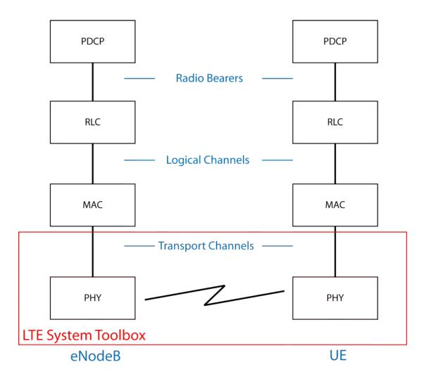
The LTE System Toolbox product focuses on the physical layer, which is highlighted in red in the preceding figure, but also supports interfacing with portions of the RLC and MAC layers, which are highlighted in blue. The primary features of the LTE physical layer are OFDM modulation, including the time-frequency structure of the resource blocks, adaptive modulation and coding, hybrid-ARQ, and MIMO.
