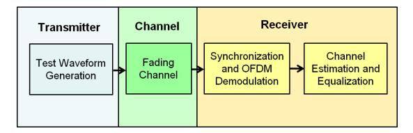
Generate an E-UTRA test model (E-TM) configuration. Use this configuration to generate the waveform and populate the resource grid.
