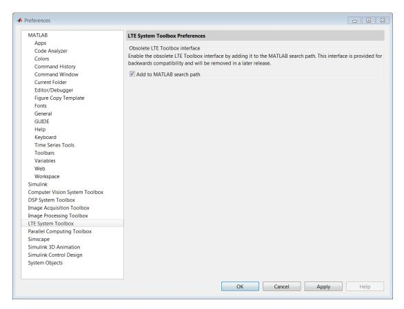
To enable the Obsolete LTE Toolbox interface, select the **Add to MATLAB search path** check box . This setting is the default and is equivalent to running the addlteobsolete function. To disable the Obsolete LTE Toolbox interface, clear the **Add to MATLAB search path** check box . This setting is equivalent to running the rmlteobsolete function. Use these functions to modify the product preferences programmatically; do not use the setpref function.
